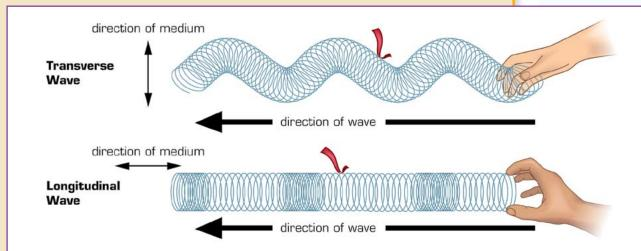
In the transverse wave (top), the wave moves from side-to-side. You can see this movement if you watch the ribbon tied to the coiled wire. In the longitudinal wave (bottom), the wave moves back and forth. You can see this movement if you watch the ribbon tied to the coiled wire.
