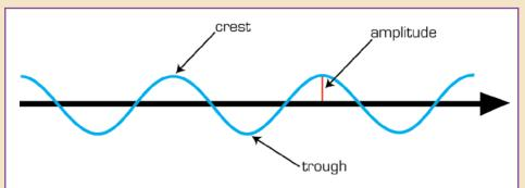
In addition to crest and trough, a wave also has amplitude. In a transverse wave, amplitude is the height of a crest. In a longitudinal wave, amplitude is how compressed the compressions are.
