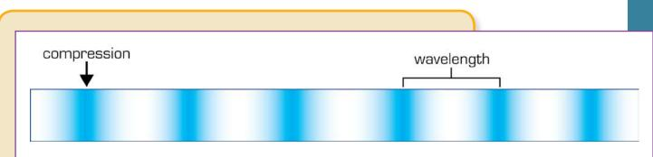
In a longitudinal wave, a wavelength is the distance between one compression and the next compression.
